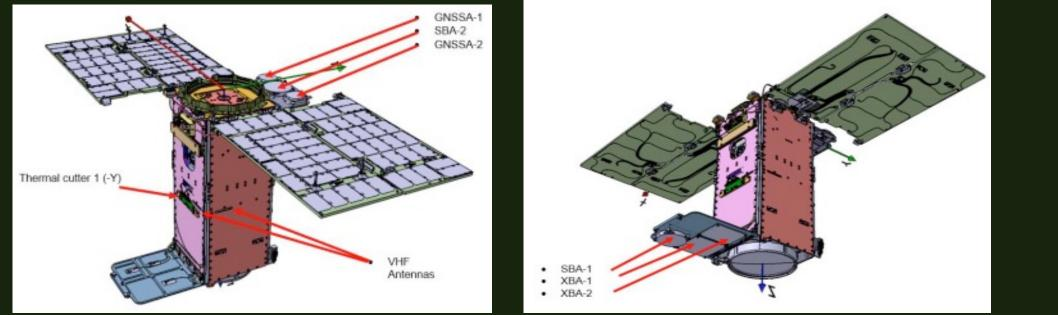
**Nominal Mass** = 25 [Kg]; **Orbit (SSO);** Altitude between 467 [Km] and 525 [Km] (Nominal); Local Time interval 09:30 to 11:30 i and from 12:30 to 14:30 . Ascending and descending.
